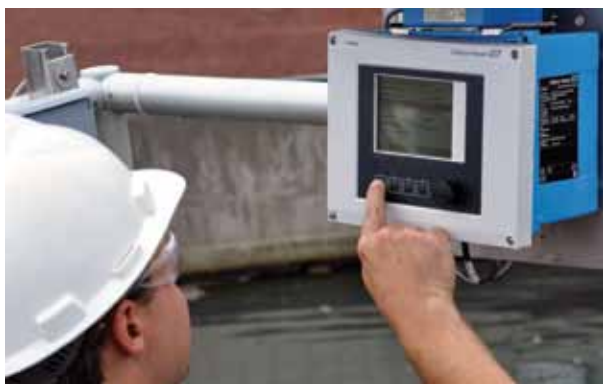
Figure 2: A multi-channel transmitter, such as this Endress+Hauser CM444, can take three pH sensor inputs and average the two closest readings.
