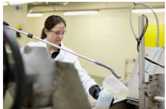
Figure 1: Technician taking a sample for comparison in the lab. She better hurry, because if it cools off the pH reading may change.
